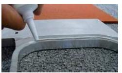
3. Smooth out the bead with your finger to assure complete and level adhesive coverage.
