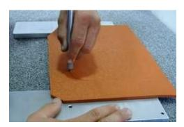
2. Continue with removal of the outside waste piece. Keep the blade **perpendicular** to the plate and follow around the outside edge of the sealing surface of the carrier plate.
