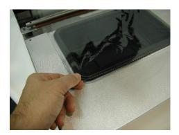
6.3 In two steps, lower the heater platen until it contacts the tray and then, in a quick downward motion, compress the heater platen down and hold down for the desired dwell time.
