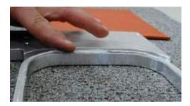
4. Lay the cut out piece (or pieces) of silicone gasket on to the sealing surface of the carrier plate. Be careful not to push down the gasket with your fingers. This will cause high and low spots on your new gasket.
