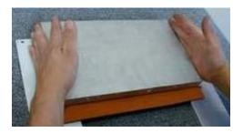
6. Stack an extra metal plate or heavy book on top of the carrier plate and let sit for at least 4 hours. Cure time may very, depending on room temperature.
