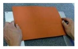
5. Using a large, heavy and flat object, lay it on top of the new gasket and push down evenly, causing any excess silicone adhesive to squeeze out the sides.
